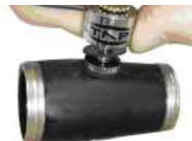
\*\*\* Drill hole 5.2mm on the barrel. Make the threading with {M6} hand tap cutting tool. Finish the edges of the hole with rasp. Screw the Adapter into the threading. Put the rubber ring on the Mic-sensor. Screw with care the Mic-sensor into the adaptor. Twist the cable on the barrel for protection.
