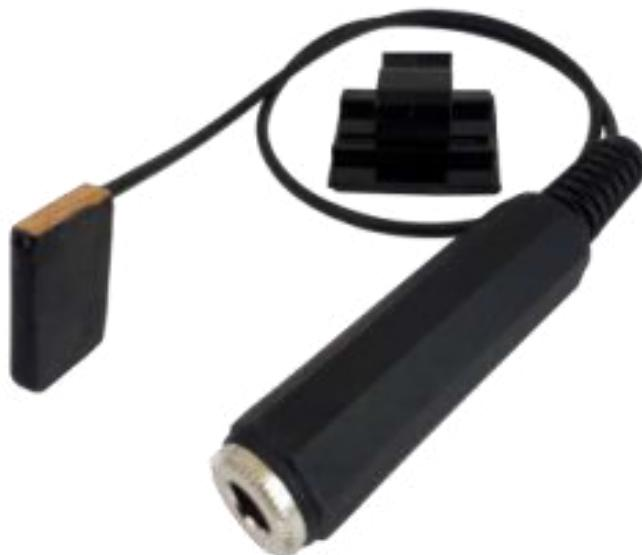
TAP sensor, is a completely special system for Double Bass and Cello. The transducer piezo-element is embedded in a piece of rubber and wedged under the bridge wing. The sensor are positioned on bridge - so that the vibrations from both the strings and the body of the instrument can be captured accurately. Different sounds can be achieved by connection. It is not necessary to use a pre-amp.
